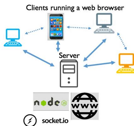
Figure 1. Typical communication in a node.js / socket.io network
